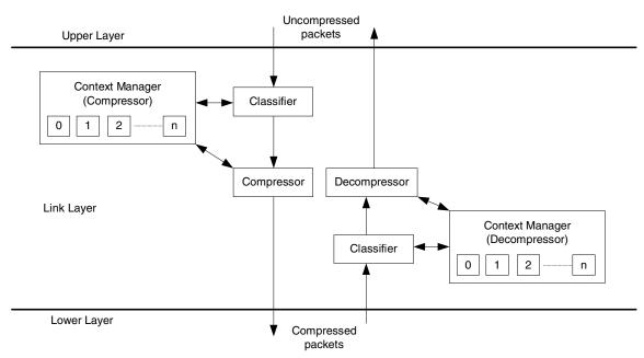
Figure 3. Header Compression Functional Blocks
