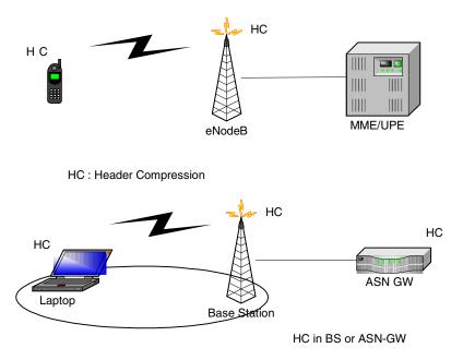
Figure 1. Header Compression in LTE and WiMAX Equipment
